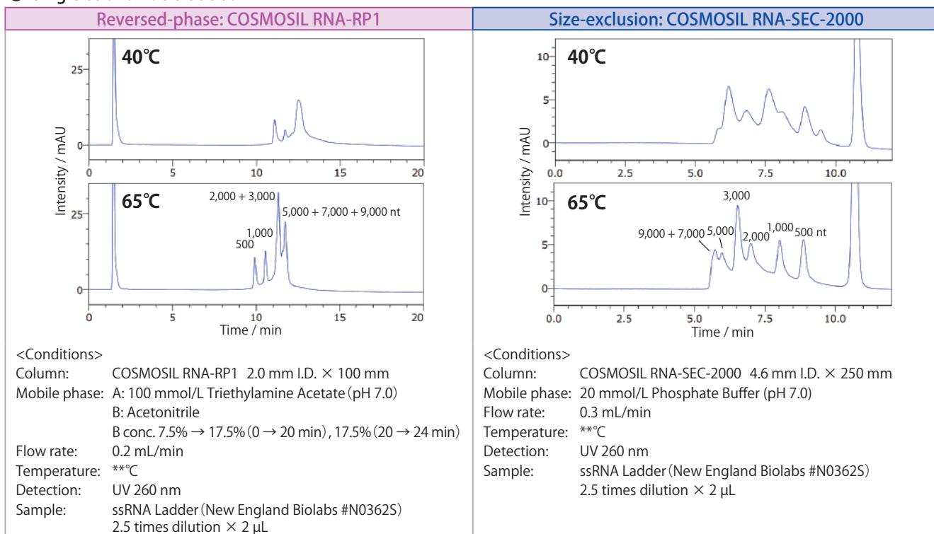
At low temperatures, single-strand nucleic acids tend to form higher-order structures, resulting in broad peaks. This may be improved by analyzing at higher temperature.
