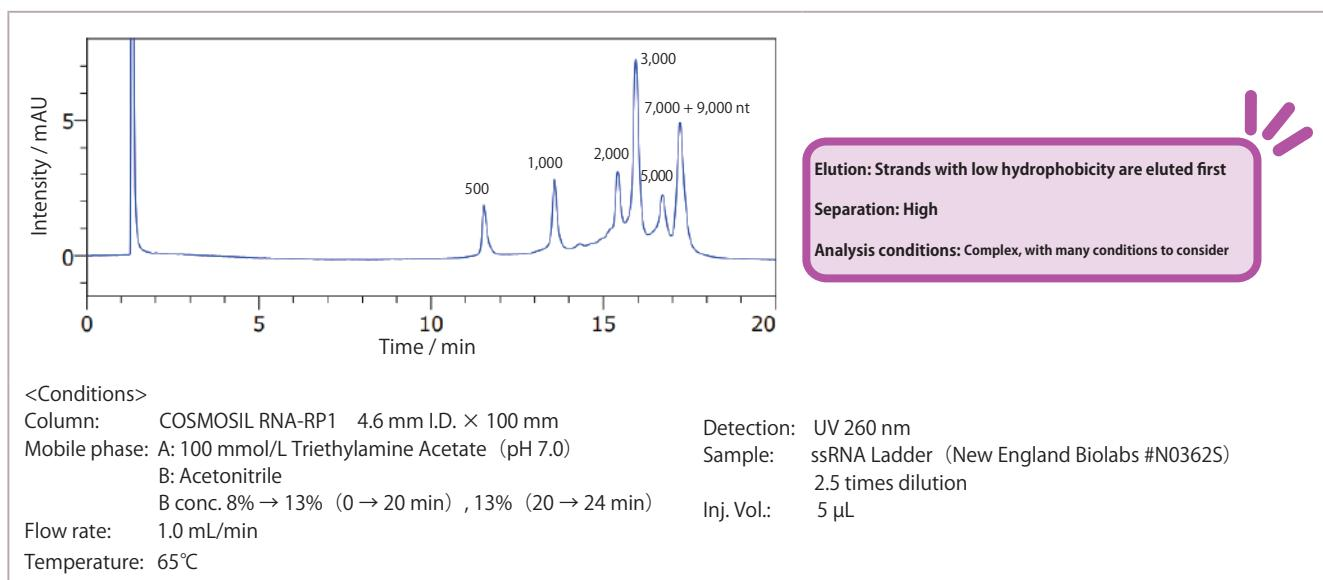
As the hydrophobicity of RNA strands generally increases with length, long strands are typically eluted after short strands. However, the hydrophobicity also differs by sequence, so it is not necessarily the case that strands are eluted in order of length. By optimizing the analysis conditions, it is possible to improve separation. For example, it is possible to adjust the mobile phase, temperature, and gradient slope. See the references on page 8 for details.
