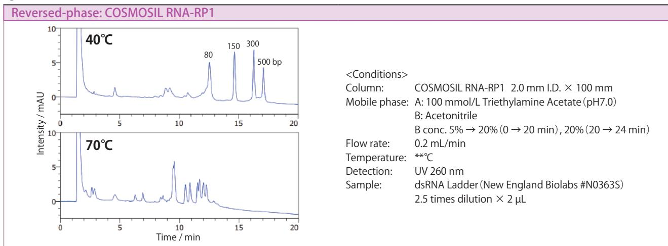
For analyzing double-strand nucleic acids in their nondenatured state, care is required when setting analysis temperature, as the strands tend to dissociate at high temperatures. Around the dissociation temperature, small differences in temperature can lead to very different separations. See the references on page 8 for details.
