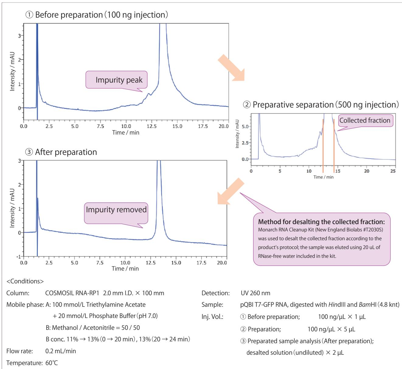
For this analysis, in vitro transcribed long-chain ssRNA (4.8 knt) precipitated using lithium chloride was used as the sample. When the long-chain ssRNA was analyzed using electrophoresis, the impurity was not detected (see page 6); however, using COSMOSIL RNA-RP1, a peak of an impurity thought to be of different length was detected (see chromatogram ① above). Using preparative separation by HPLC, the impurity peak was successfully removed (see chromatogram ③ above).
