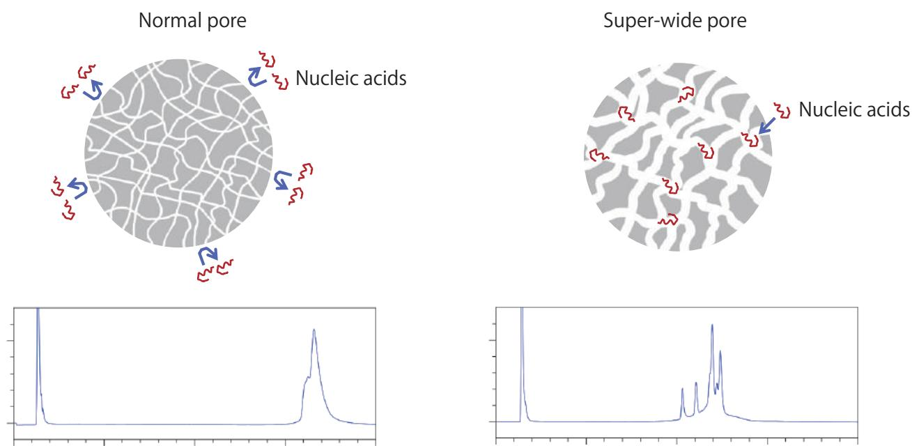
HPLC columns for general use typically have silica gel with an average pore size of 8 to 12 nm, whereas COSMOSIL RNA-RP1 uses silica gel with super-wide pores.
