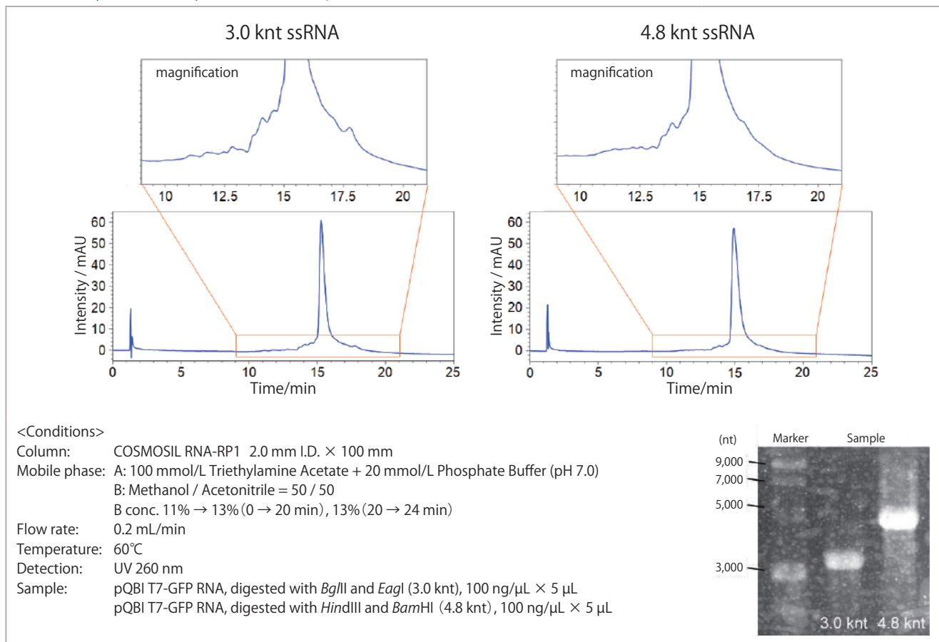
Upon analyzing long-chain ssRNA purified using lithium chloride precipitation, impurity peaks not detected with agarose gel electrophoresis were confirmed. This shows that it is possible to separate impurities in vitro transcribed ssRNA using reversed-phase HPLC. Also see page 1 for information about purification of long-chain ssRNA.
