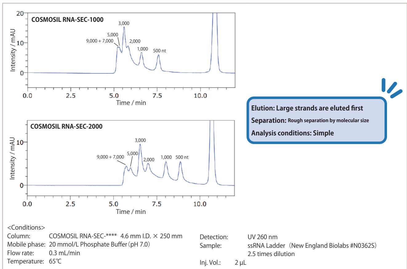
Compared to COSMOSIL RNA-SEC-1000, which has a pore size of 100 nm, RNA-SEC-2000, with a pore size of 200 nm, is suitable for analysis of large strands. Use different pore sizes depending on the strand sizes you need to separate.
