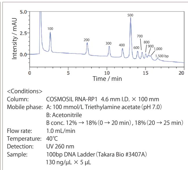
Fragments that are difficult to separate using agarose gel electrophoresis can be separated using COSMOSIL RNA-RP1. See the references on page 8 for details.
