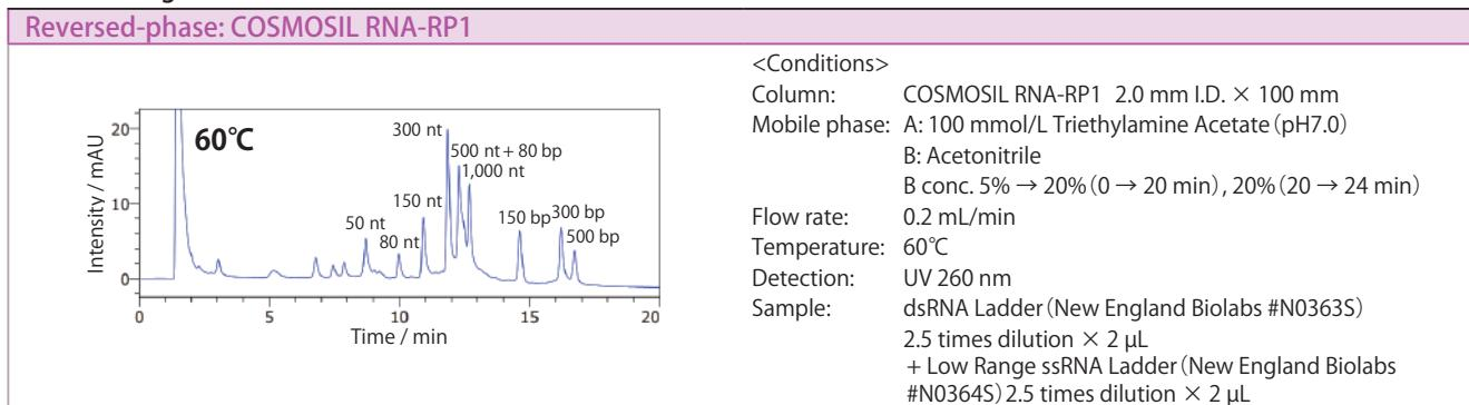
By analyzing at a temperature at which single strands do not form higher-order structures and double strands do not dissociate, it is possible to simultaneously analyze both.
